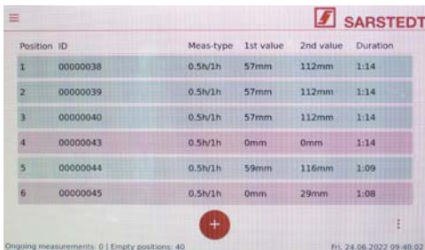
Figure 12: Starting a measurement by pressing the "+"key
