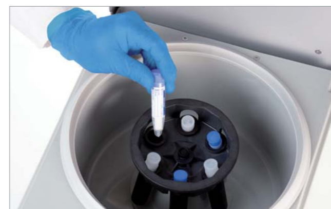
Centrifugation of Salivettes to collect saliva.
